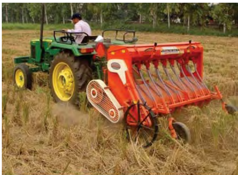
A zero-till seed drill in operation at Indian Agricultural Research Institute farm.
