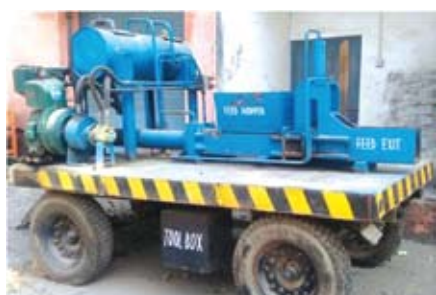
IC engine operated, tractor trolley mounted hydraulic plunger/piston press type feed block making machine
