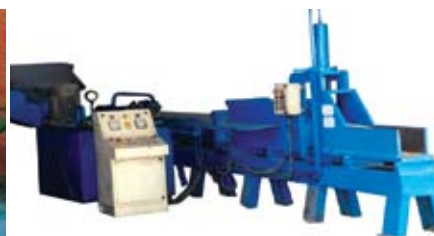
Electrically powered hydraulic plunger/ piston press type feed block making machine
