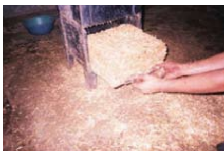
Manually operated feed block making machine
