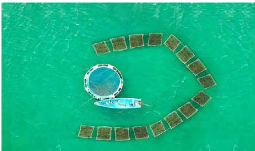
Seaweed rafts integrated with cobia cage (IMTA)
